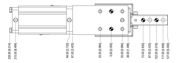
THIS SHEET IS FOR 75mm STROKE DETENT OPTION ONLY
